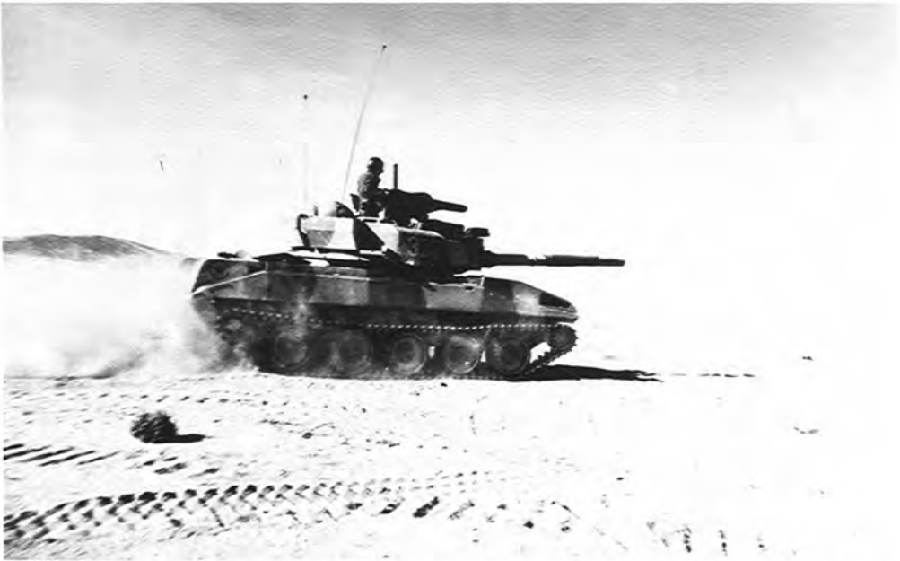
An M551 Sheridan Light Tank is visually modified to resemble a Soviet T-72 main battle tank. These VISMOD vehicles, used by the OPFOR, added realism to maneuvers.
