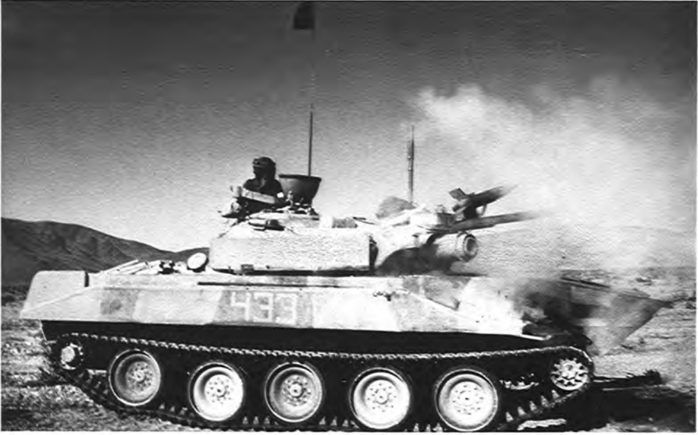
An M551 Sheridan Light Tank, visually modified to represent an OPFOR BMP Fighting Vehicle, fires a 73-mm. smooth bore cannon at U.S. forces, while its SAGGER antitank missile is readied to attack the next target. The real BMP was a smaller vehicle with a lower silhouette.
