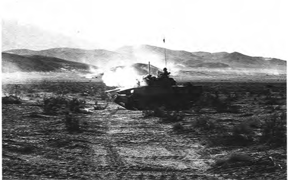
A BMP fires its 73-mm. smoothbore gun at a U.S. Army armored vehicle in the Valley of Death. The smoke from a Hoffman device indicates the gun's firing, while a MILES emitter records hits, kills, or near misses on the target.
