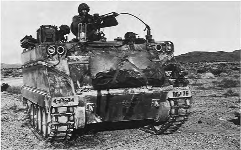
A mechanized infantry squad mounted in an M113 Armored Personnel Carrier moves to contact with the OPFOR. Visible along the side of the APC is a belt of MILES sensors to register incoming hits. The strobe light to the gunner's right is activated when a hit is registered.
