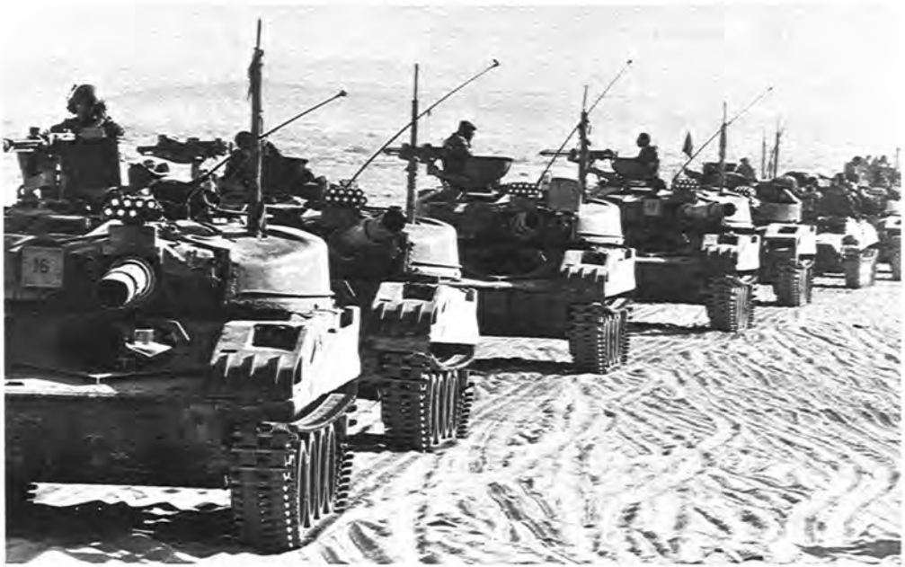
An OPFOR column heads for battle in its "VISMODed" T-72 tanks. The data transmitter antennas will relay battle hit and kill data to the NTC core instrumentation facility.
