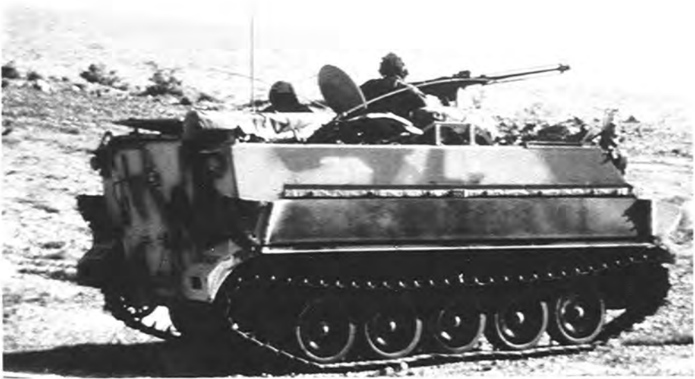
An M113A1 armored personnel carrier moves to the attack. The MILES sensor belts are attached to the side, and a kill indicator light is mounted on the right of the vehicle.
