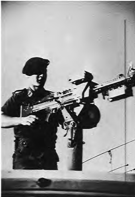
An OPFOR soldier mans a MILES-equipped M60 machine gun, modified to resemble a Soviet 12.7-mm. heavy machine gun, atop a BMP vehicle.
