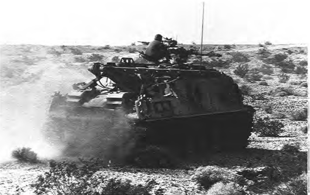
An armor soldier moves his huge M88 recovery vehicle into a battle position. The M88 crew recovered damaged or immobile tanks, APCs, and self-propelled howitzers.
